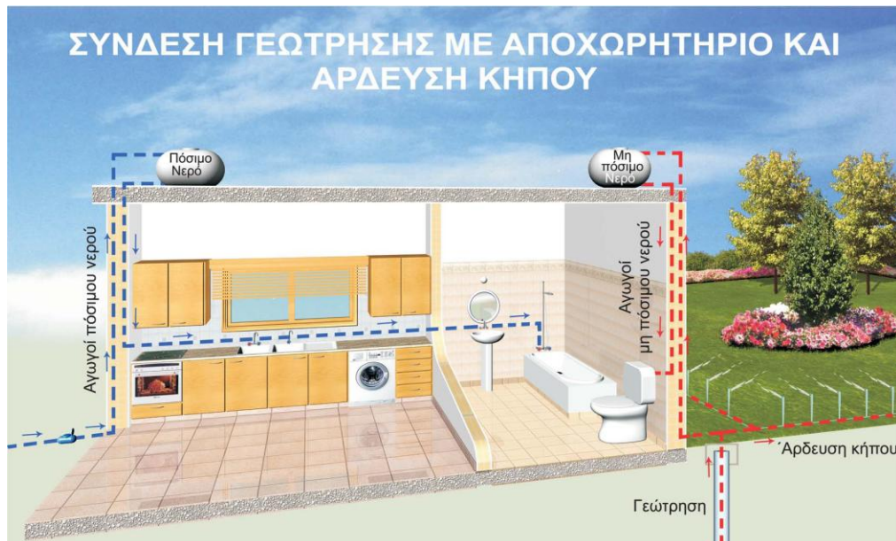
Photo 6: Connection of borehole to garden and toilets
