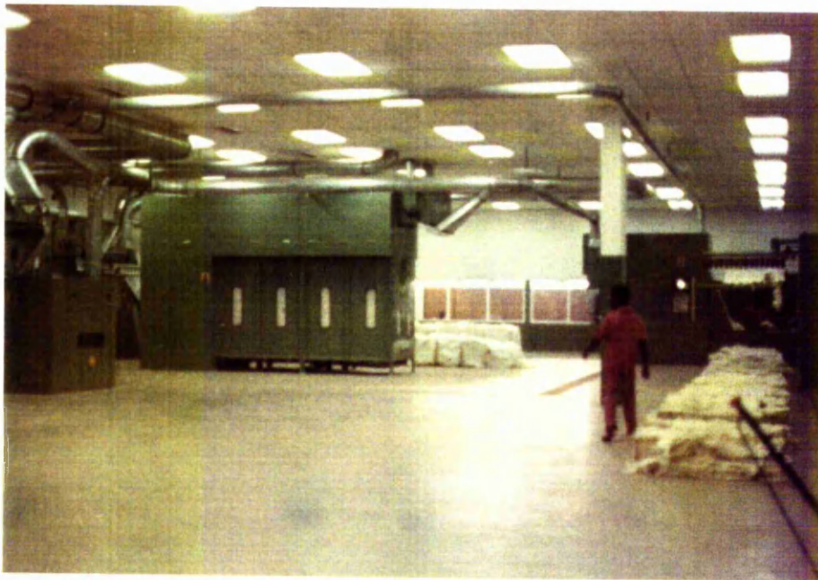
Figure 4.2. Automatic Bale Plucker/Feed
