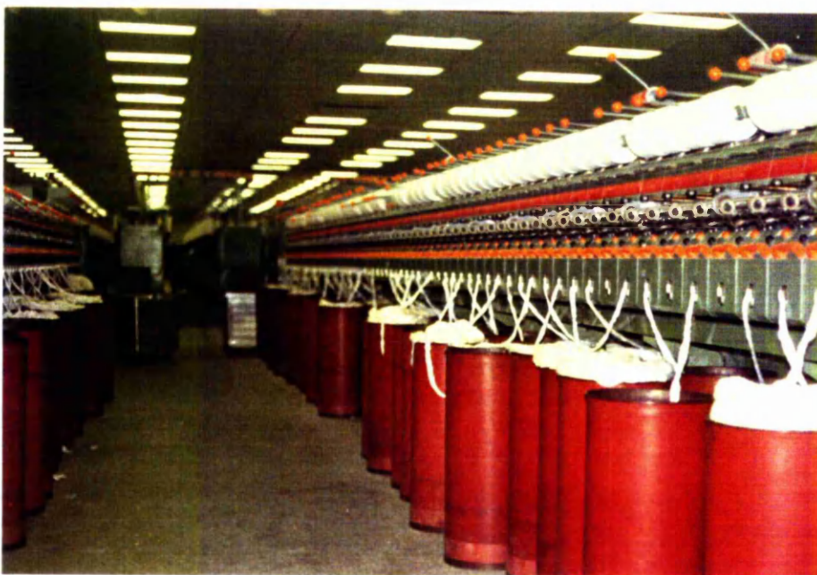
Figure 4.5. Rotor or Open-End Spinning
